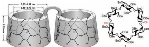
Figure 1. (a) Dimensions of dimeric CDs from \alpha -, \beta -, or \gamma -CD (left). (b) Structure of C 2 symmetrical 6 A ,6 D -diol ( 1 ) of \alpha -CD used for synthesis (right).
